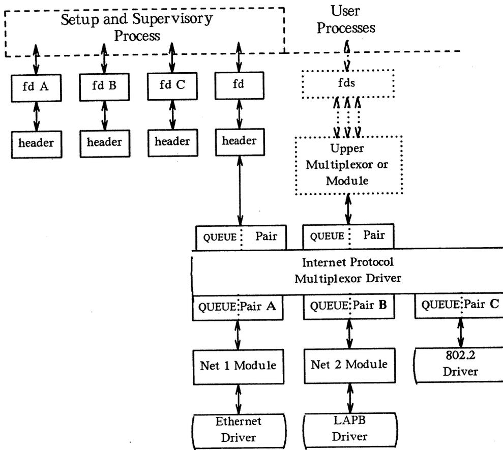
Figure 12-2. Internet Multiplexor After Connecting
