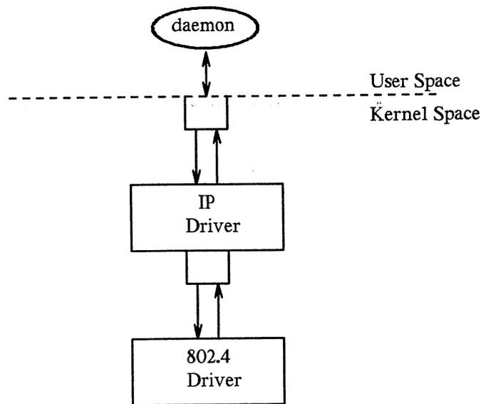
**Figure 4-6.** IP Multiplexor After First Link
