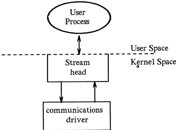
Figure 2-1. Stream to Communications Driver
