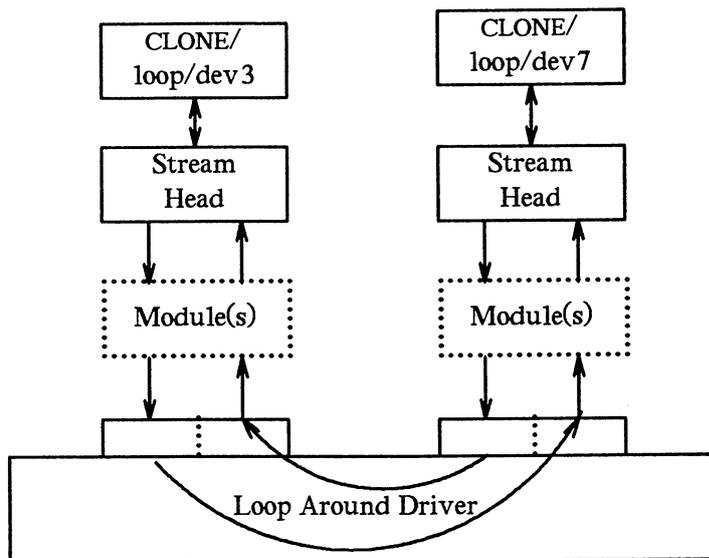
Figure 11-1. Loop Around Streams
