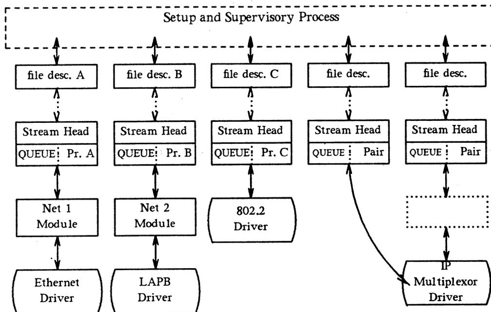
Figure 12-1. Internet Multiplexor Before Connecting
