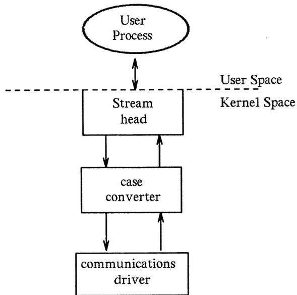
Figure 2-2. Case Converter Module
