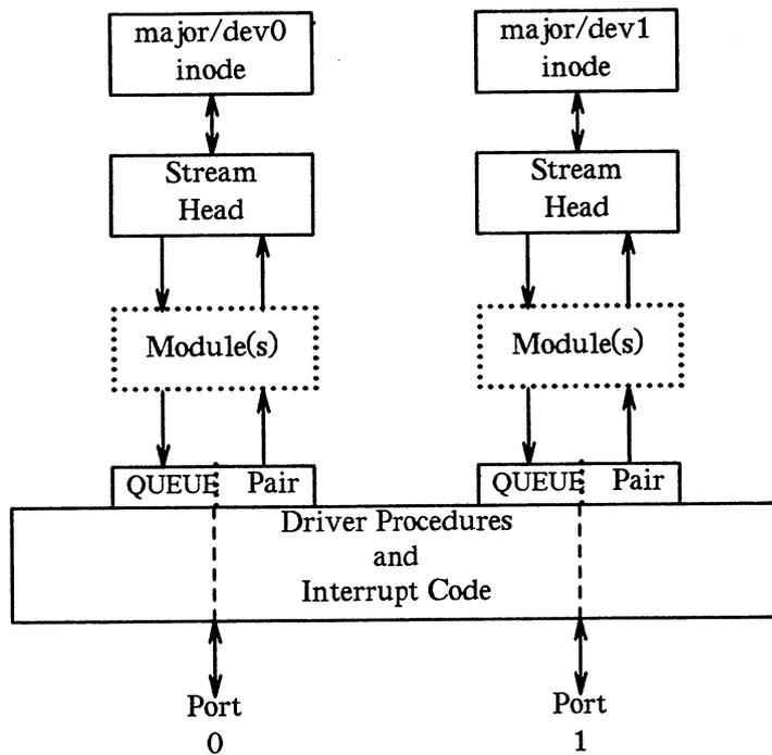
Figure 10-1. Device Driver Streams
